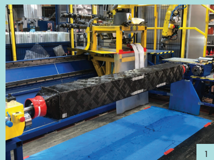
1 / Advanced winding of beam with carbon sensors integrated
