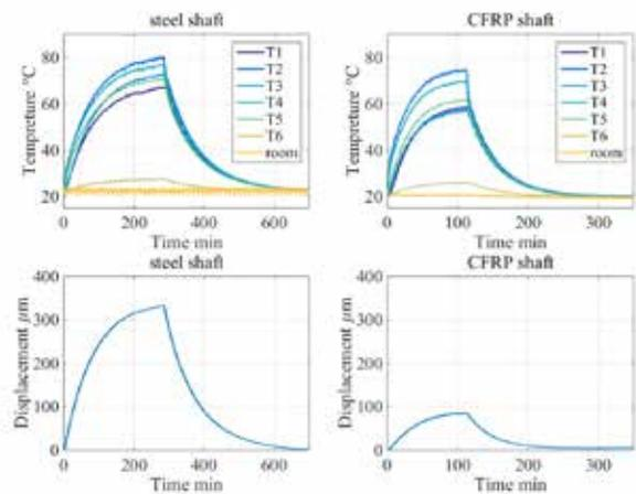
Comparison of steel and carbon spindle. Temperature measure along the spindle and resulting displacement over time.
