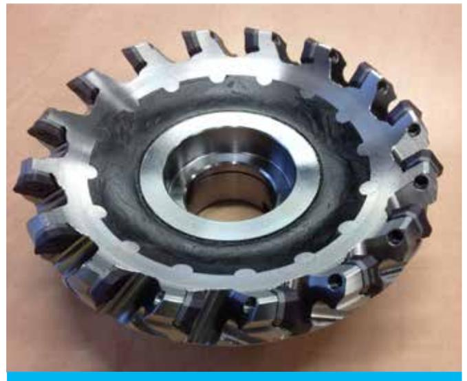
The hybrid milling tool is produced by depositing carbon and graphite fibre onto a steel part using a process called robot assisted filament laying (RAFL). The steel body acts both as a mandrel and as a means of connecting the tool to the tool holder and the tool holder to the spindle. It also provides a means for the attachment of the tool to the milling teeth.
